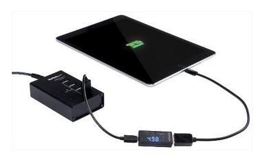
between showing the voltage and the current, so you can keep an eye on both measurements without having to adjust the tester.
