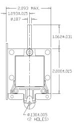
Solenoid shown energized with plunger fully seated in extended position
