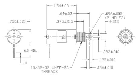
Solenoid shown energized with plunger fully seated Supplied with mounting bracket, hex nut and lock washer shipped loose
