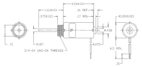
Solenoid shown energized with plunger fully seated in extended position Supplied with mounting bracket, hex nut and lock washer shipped loose
