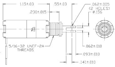
Solenoid shown energized with plunger fully seated Supplied with mounting bracket, hex nut and lock washer shipped loose
