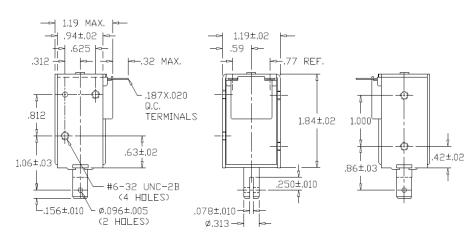
Solenoid shown energized with plunger fully seated
