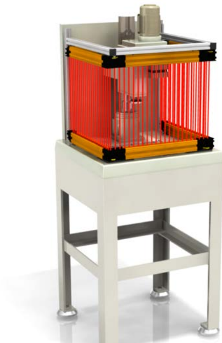
Figure 43. Cascaded light screens guarding a u-shaped cell
