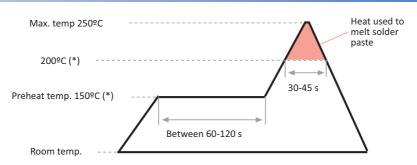
(\*) Melting point temp. depends on solder properties
