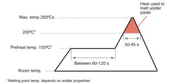
This reflow profile is provided as a guideline. Optimal profile may differ due to oven type, assembly layout or other design or process variables. Customers should verify actual device performance in their specific application and reflow process.
