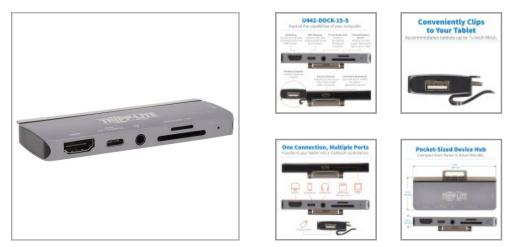
USB-C dock clips to your iPad Pro, tablet or smartphone to add 4K HDMI, USB-A, PD Charging and memory card slots to its USB-C port.
