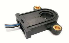
The PST-360 through hole / hollow-shaft position sensors combine three critical design features; 1) through hole where the shaft passes through the sensor, 2) high accuracy absolute position feedback over up to 360 degrees, and 3) a true non-contacting sensing element. Piher's design does not rely on gears or other rotating parts.
