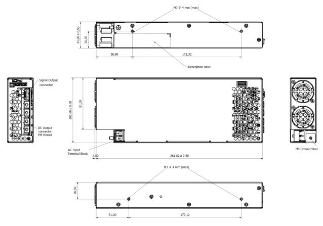
Figure 7. Mechanical Drawing - MBE1200-1T24 / MBE1200-1T48 Models
