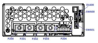
Figure 9. Rear View - MBE1200-1T24 / MBE1200-1T48 Models
