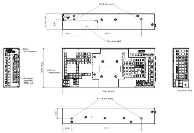
Figure 4. Mechanical Drawing - MBC1200-1T24-PCF Model
