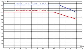
U-Chassis and Perforated Cover Forced Air Cooling (Models MBC1200-1T24-UCF / -PCF) Air flow from AC side, V1 nominal
