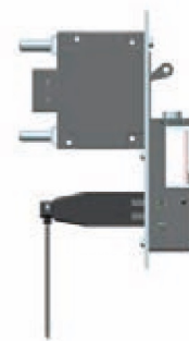
RBR returns to initial configuration (by gravity)
