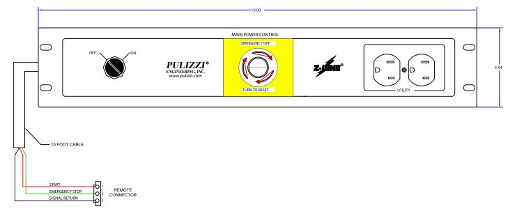
RACK MOUNTED STEEL CHASSIS GREY FED STD 595-26559
