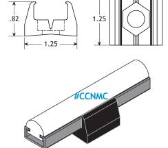
PLASTIC CLIP FOR "A" SIZE MOUNTING CHANNELS #CCNMC (Mounting Channels see pg. 40) Tightens w/ #28 Plastic Knob and 5/16-18 S.S. Hex Bolt
