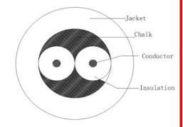
Cable Marking: 1PR 20AWG 001M…100M
