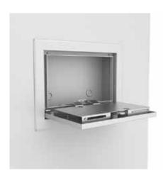
**Description:** Horizontal hinged keyboard tray with lateral sliding mouse pad (L.H, or R.H.). Equipped with panel stay. When the tray is folded out, the enclosure is sealed for dust ingress by a closed chamber.
