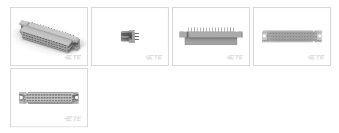
Connector & Housing Type: Receptacle Connector System: Board-to-Board Termination Post & Tail Length: 3.3 mm [.13 in] Number of Positions: 48 Centerline (Pitch): 2.54 mm [.1 in]
