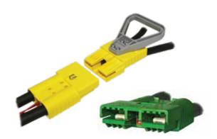
SBE° and SBX° connectors can integrate up to 8 auxiliary power / signal contacts along with the two primary power circuits. Sequencing within auxiliary positions is possible using the 4 pin lengths available in the 1x4 auxiliary connector. SBE° and SBX° offer touch safe housings.
