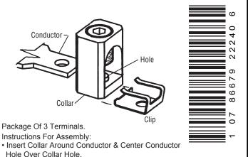
• Install Clip with Legs on Top of Conductor & Snap Its End
