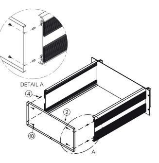
2. Insert <sup>(1)</sup> Nut OB M3 [4] into the rail slot on side frame then install <sup>(2)</sup> inside front panel by
