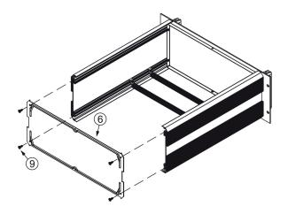
4. Install (a) rear panel cover and tie with (c) Umbrella Phillips screw M3x6 (Dog Point) [4]. [Convex shape is outside, see detail A in item 5].
