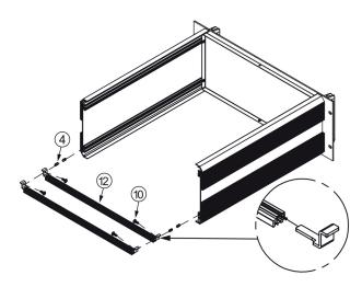
3. Insert <sup>(1)</sup> Nut OB M3 [4] into the rail slot on side frame at the bottom. Install <sup>(2)</sup> GP Bar [2] with
