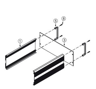
Install (5) AL handle and (3) AL front panel to (1) side frame with (8) Hex socket screw M5x20 [4].
