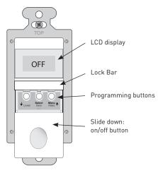
To access RT-100 setup buttons, gently pull the Lock Bar away from the switch face and slide the on/off button down.
