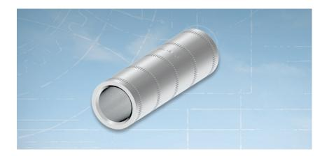
TE's Dual Rated Aluminum Crimp Splices are designed on high conductivity aluminum. The Dual Rated Aluminum Crimp Splices are electro-tin plated to resist electrolytic corrosion. They are suitable in applications from 600 V to 35 kV.
