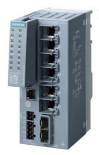
SCALANCE XC206-2SFP G managed Layer 2 IE switch; IEC 62443-4-2 certified; 6x 10/100/1000 Mbps RJ45 ports; 2x 1000 Mbps SFP; 1x console port; diagnostics LED; redundant power supply; temp. range -40 °C to +70 °C; mounting: DIN rail/S7 mounting rail/wall; redundancy functions; Office features (RSTP, VLAN,...); PROFINET IO device; Ethernet/IP-compliant; C-plug slot;
