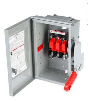
Siemens Low Voltage Circuit Protection Heavy Duty Safety Switches. Type: ENCLOSED, SAFETY SWITCH Std: UL V. Rating: 600V A. Rating: 60A No. Of Poles: 3P F. Rating: 60Hz Action: SINGLE THROW Material: 304SS Enclosure: TYPE 3R. 2-3 point mounting holes. O. Cycles: 10000 O. Temperature: (-20F-120F) AMBIENT TEMPERATURE Environmental Conditions: OUTDOOR
