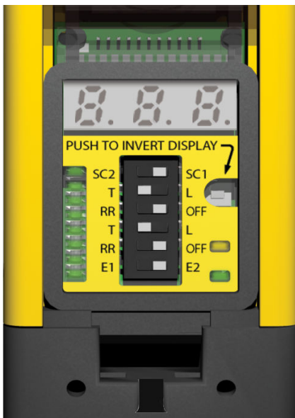
Figure 24. EZ-SCREEN Configuration DIP Switches (Receiver)
