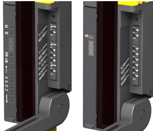
Figure 39. Accessing the configuration switches
