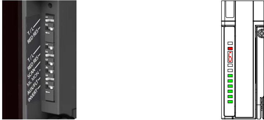
Figure 20. DIP switch settings to program mute configuration options
