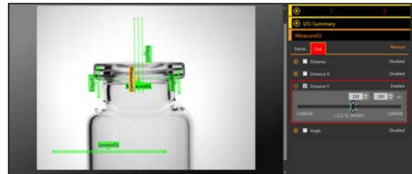
Figure 220. Bad Part—Missing Stopper
