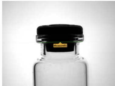
Figure 216. Measure Tool from Edge02 to Edge03
