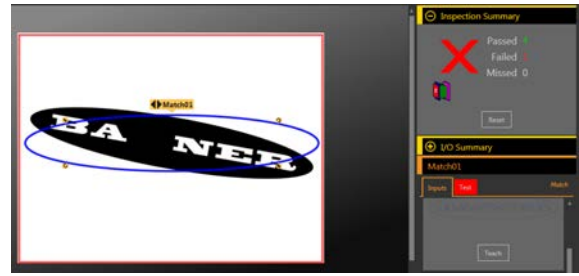
Figure 243. Bad Part—Missing Letter
