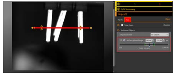
Figure 263. Bad Part—Bent Pin
