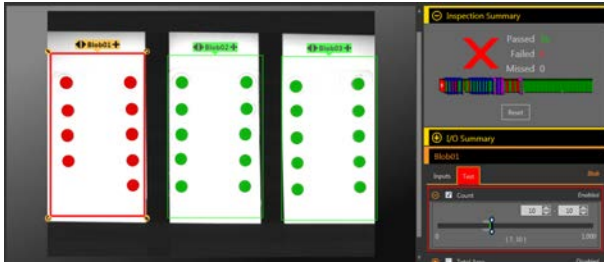
Figure 142. Bad Part—Missing Pill
