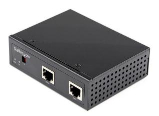
Splits a PoE connection (max 90W) into separate data (RJ45) and DC power (terminal block) that can power any device that uses DC power between 12V-48VDC (1.5A). Power non-PoE devices using network infrastructure, where power is not available.
