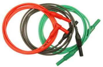
These single test leads have either a 4mm plug or a 90° 4mm plug at either end. The cable is silicone and the total length is 1.5m. Plugs are rated 10A. 1KV CAT III
