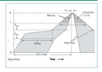
Note: All temperatures refer to topside of the package, measured on the package body surface.
