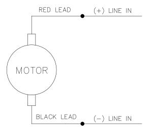
CONNECTIONS SHOWN FOR CCW ROTATION FACING LEAD END OF THE MOTOR
