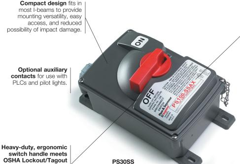
Nonconductive, watertight, corrosion, heat, and impact-resistant thermoplastic enclosure ensures NEMA 4X and 12 ratings. Withstands the harshest industrial environments.
