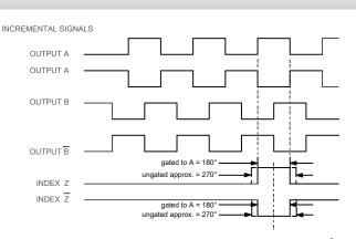
CLOCKWISE ROTATION AS VIEWED FROM THE SINGLE WHEEL SIDE NOTE: ALL DEGREE REFERENCES ARE ELECTRICAL DEGREES WAVEFORM SHOWN WITH OPTIMAL COMPLEMENTARY SIGNALS A, B, Z FOR HV AND OD OUTPUTS ONLY
