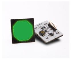
RGB LED illumination provides a high brightness user touch area with unmatched uniformity of Illumination. The solid-state switch design has a non-latching output of 40mA maximum operating from a supply voltage of 6VDC to 28VDC. The 35mm version offers designers adjustable low, medium and high touch sensitivity to suit the application. The operating temperature of the switch modules is 0° to 50°C
