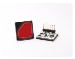
TT Electronics provides market leading 'off the shelf' LED Backlit Capacitive Switch Modules in component form which allow designers to evaluate touchscreen technology and even manufacture simple control solutions.
