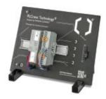
PLCnext Technology starter kit including AXC F 2152 PLCnext Control device, AXL Smart Elements DI16/DO16/ Al4 I/O modules, slide potentiometer, pushbuttons, power supply unit, and patch cables.
