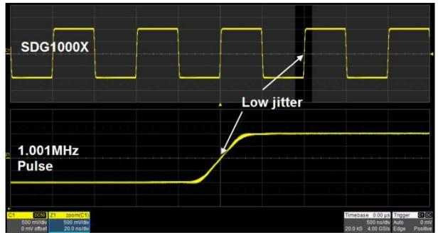
When a Pulse waveform is generated by a common DDS generator, there will be a one-clock-jitter if the sampling rate is not an integer-related multiple of the output frequency. RSDG1000X EasyPulse technology successfully overcomes this weakness in DDS designs and helps to produce low jitter Pulse waveforms.
