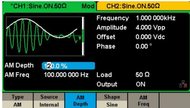
Multiple modulation types: AM, DSB-AM, FM, PM, FSK, ASK, PSK and PWM.
