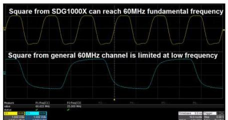
Benefiting from a special square-wave generating circuitry, the Square from the RSDG1000X breaks the 60 MHz bandwidth barrier, reaching rise/fall times of less than 4.2 ns, and frequencies up to 60 MHz.
