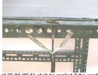
The connection shall not break under a pull applied for 1 minute between the element and the conductor before the element has been assembled into the fittings...
