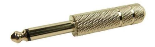
A 1/4" screened Mono Jack Plug. Metal body. Rivetted construction. Maximum cable Ø6.4mm with grommet removed Jack Plugs are manufactured from solid nickel-plated brass with high temperature Phenolic / PBT insulators. The cable clamp, which is an integral part of the ground screen contact, clamps firmly without damaging the cable.
