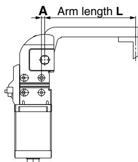
\* Arm length "L" indicates the distance between the clamp arm shaft and the clamping position.
