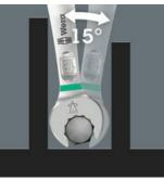
The Joker 6003 ring spanner with its special mouth geometry mouth side pivoted by 7.5° and the double hexagon profile doubles the placement possibilities when repeatedly turning the wrench 180° around the longitudinal axis. Bolts and screw heads can be "accessed" every 15°. The Joker 6003 will automatically find the respective placement point after every turn.
