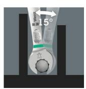
The Joker 6003 ring spanner with its special mouth geometry mouth side pivoted by 7.5° and the double hexagon profile doubles the placement possibilities when repeatedly turning the wrench 180° around the longitudinal axis. Bolts and screw heads can be "accessed" every 15°. The Joker 6003 will automatically find the respective placement point after every turn.
