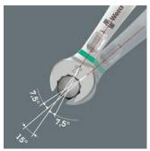
Thanks to the mouth side pivoted by 7.5°, double hexagon geometry and an adjusted application method (placement - screwdriving - turning - replacement screwdriving - turning, etc), even screwdriving challenges allowing a pivoting angle of less than 30° can be solved. **Double-hex geometry**
