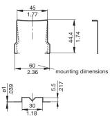
Retaining clip for circuit breaker 2210 recommended for fitting single pole devices Y 302 974 21
