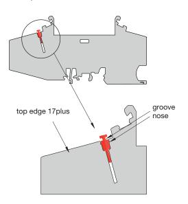
When mounting several modules side by side, proper insertion of the 32 A busbar X 222 005 01/02/03 has to be observed, i.e. the busbar must be pushed in evenly across the whole length from left to right, repeatedly if necessary. The groove of the busbar must be flush with the top edge of the Module 17plus.
