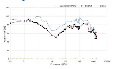
Test performed with a two-coat thickness.
