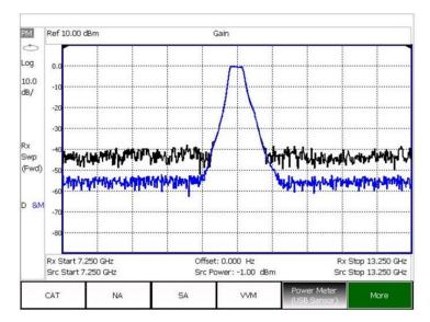
Measured using U2021XA power sensor
