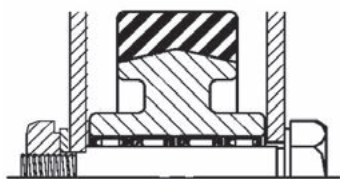
Fig. B3-7. Clutch and bearing arrangement for heavy loads
