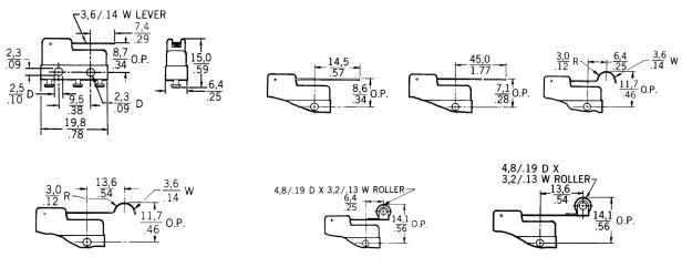
NOTE: The two mounting holes accept pins or screws of 2,21 mm (0.087 in) maximum diameter
