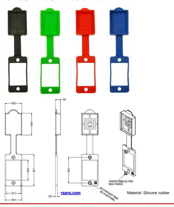
This range of gaskets fit most of our Slim feedthrough connectors. They function as dust seals and for colour identification. Useable on plastic and metal models. They are all supplied with brass spacers. Using spacers can improve the sealing function and fit. Available in 4 colours.
