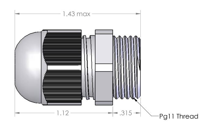
LOCK NUT INCLUDED BUT NOT SHOWN NO O-RING IS NECESSARY TO OBTAIN IP68 SEAL. CRUSH RIBS ON THE UNDERSIDE OF HEX WILL PROVIDE THE SEAL.
